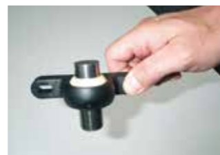
Tolerance test with plug gauge
