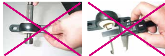
Inadequate test equipment; plug gauge too short Wrong test equipment; caliper
