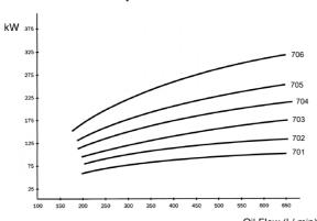
Oil Flow (I / min) Graphs were plotted using the parametres shown in the right side table. For oil pressure drop graphs see separated sheet.
