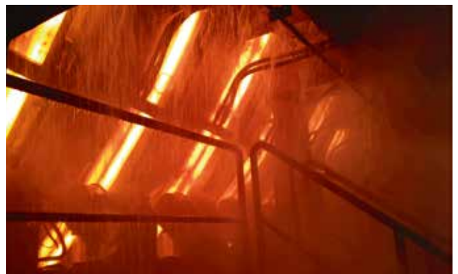
Secondary cooling zone of billet caster
