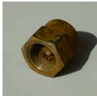
Clogged vane of a full cone nozzle
