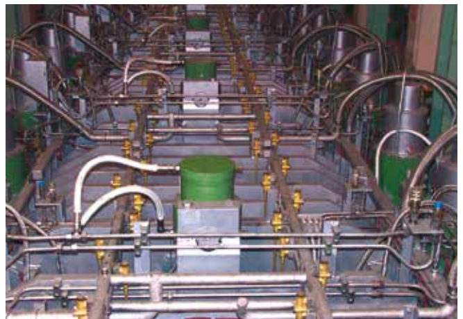
Horizontal segments with Mastercooler SMART nozzles
