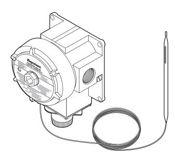
This EEx d approved surface sensing thermostat provides temperature control for all Raychem BTV, QTVR, KTV, VPL and XTV heating cables in hazardous areas. The switching temperature range is -4°C to +163°C and is adjustable externally to the Ex enclosure by a dial mounted under a bolted-on cover and seal.
