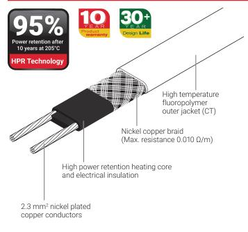
The nVent RAYCHEM HTV self-regulating heating cable is designed for freeze protection or process temperature maintenance of pipes and vessels with very high continuous operating temperatures (205°C).
