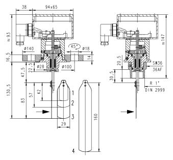
Adapt paddle 1 for DN 25. From DN 100, adapt paddle 4: DN 100 Paddle length 92 DN 125 Paddle length 117 DN 150 Paddle length 143 from DN 175 unshortened
