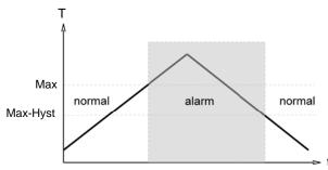
A switchover delay time ( $t_{DS}$ ) can be applied to the switchover to the alarm state. Equally, one switch-back delay time ( $t_{DR}$ ) of several can be applied to switching back to the normal state.
