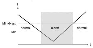
With a maximum-switch, exceeding the limit value causes a switchover to the alarm state. Return to the normal state occurs when the measured value once more falls below the limit value minus the set hysteresis.
