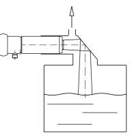
High dust levels reduce the ultrasound signal and produce incorrect measurements. Depending on density, foams may or may not be recognised.
