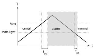
In the normal state the integrated LED is on, in the alarm state it is off, and this corresponds to its status when there is no supply volta-
